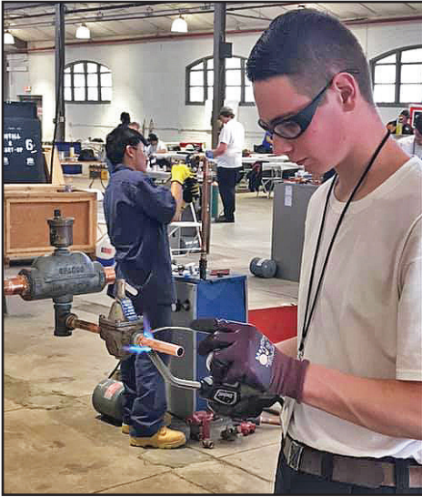
ABOVE: Jon Baker working on a weld for his hydronic heating system while participating in the state SkillsUSA Competition.
